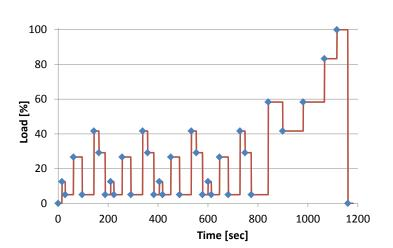
The load cycling starts with the appropriate cell leak test, break-in and conditioning as described in 3.2 and 3.3 and is performed according to the following table 2. In this specific case, a power demand of 100 % is defined as the power generated at 0.659 V at BoL (approximately 90 kW).
