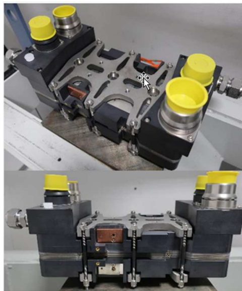
Figure 1. NM12 short stack test hardware showing end plates, clamping fixture and media interface (covered with yellow cups).
